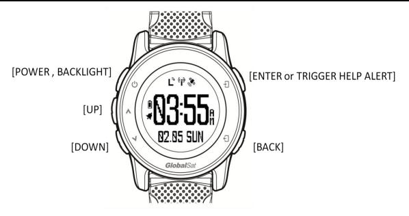
To power on/off by holding POWER button 2 seconds To Trigger help alert by holding ENTER button 3 seconds
